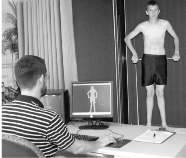
ABOVE: The 3-D body scanner resembles a dressing room. The patient stands in the center, and within 15 seconds, four eye-safe lasers and eight synchronized cameras scan the body.
